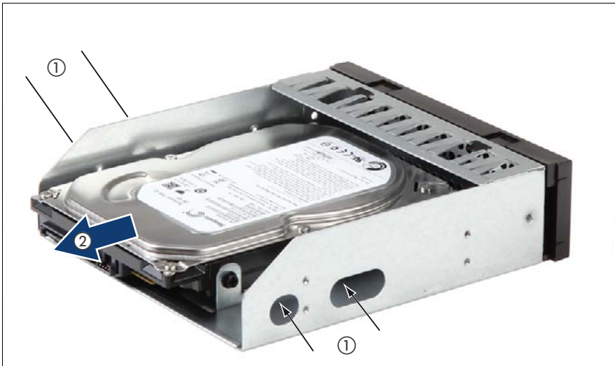
Figure 41: Removing the HDD out of the 5.25-inch dummy cover
